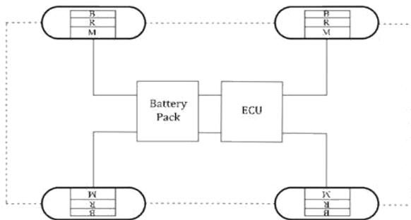
FIGURE 1: Basic structure of a hub-driven electric vehicle.
