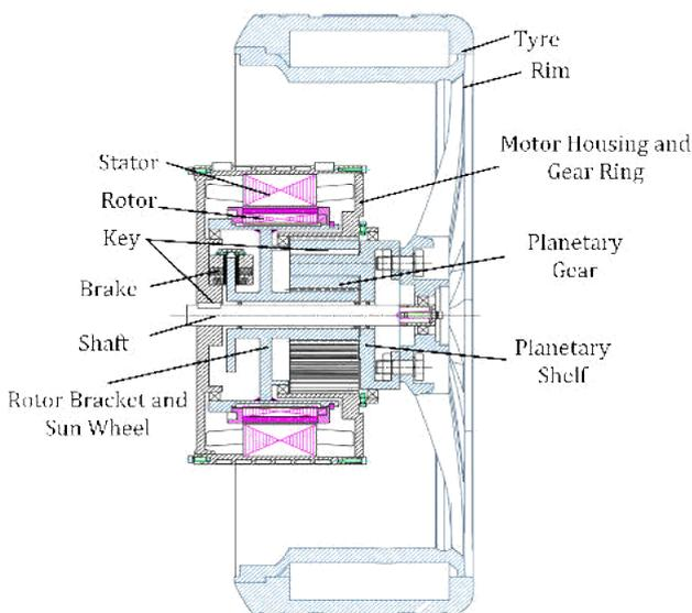
**FIGURE 2:** Structure Scheme of Hub Drive System.
