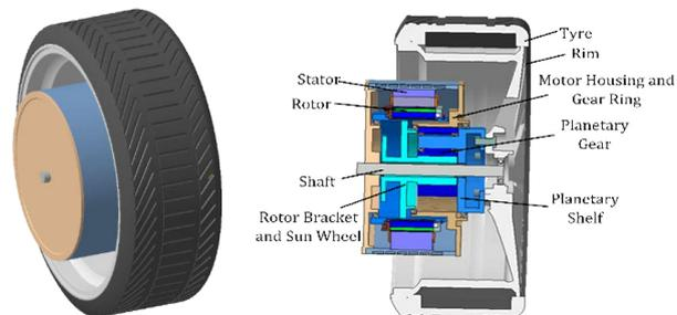
a) Overall Structure b) Internal Structure
