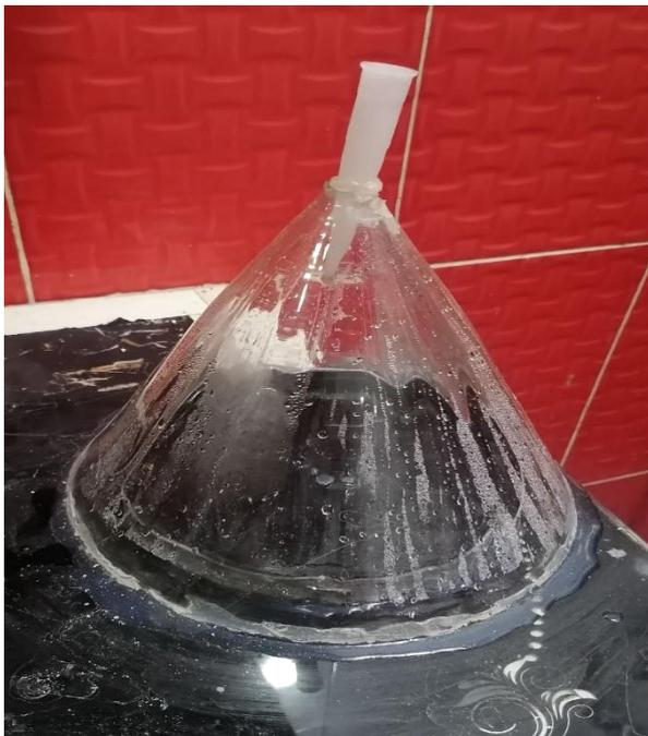
FIGURE 1: A photographic picture of the Conical Solar Still (CSS).
