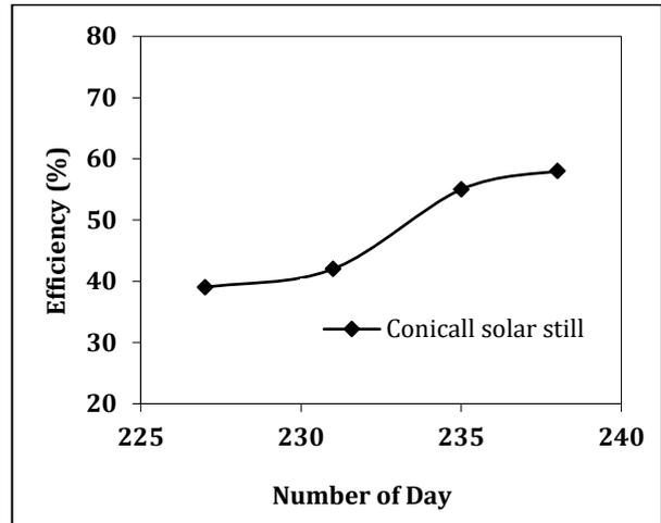
FIGURE 6: Thermal efficiency of the conical solar still through some days of (August 2023).
