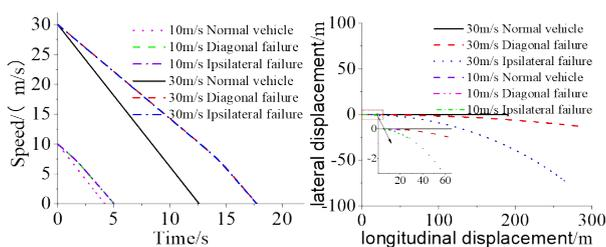
(a) Brake speed diagram. (b) Trajectory comparison diagram.
