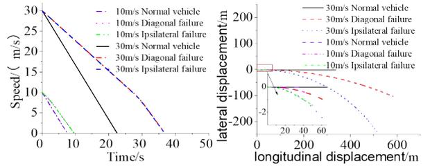
(a) Brake speed diagram. (b) Trajectory comparison diagram.
