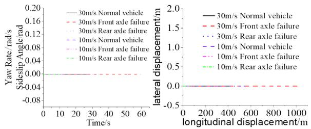
(c) Yaw rate and Sideslip angle diagram. (d) Trajectory comparison.
