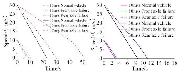
(a) Z=0.2 Brake speed diagram. (b) Z=0.8 Brake speed diagram.
