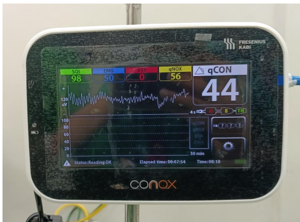
FIGURE 1: Conox Anesthesia Monitor to Measure Depth of Anesthesia and Pain Stimuli In Patients.
