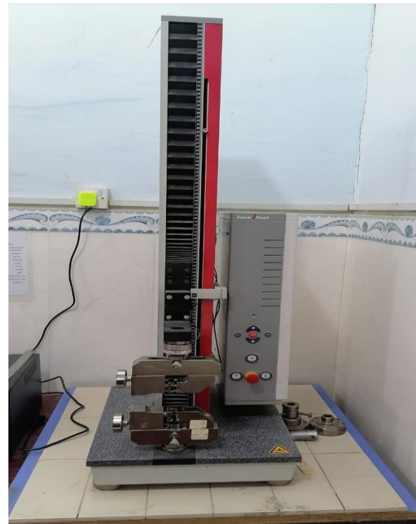
FIGURE 2: Mechanical properties measuring device (Tensile).
